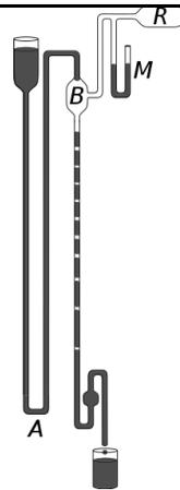
1. The Sprengel pump is a form of non-electric vacuum pump that uses drops of mercury falling through a small-bore capillary tube in order to trap air. Mercury is contained in the reservoir and flows into bulb B, where it forms drops which fall leaving air entrapped in bulb B. Mercury is collected and restored to the left reservoir. In this way almost all air can be removed from bulb B and by extension vessel R (Sella 2008).
