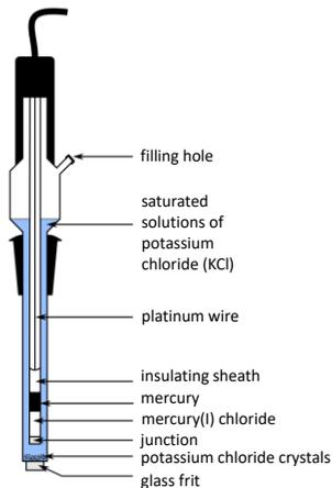
**Figure 1: Principal components of a calomel electrode (source: Wikipedia.org)**
